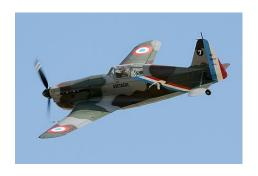
This is the Swiss version of the French M.S. 40 and M.S. 412. The most visible difference being a fixed engine coolant radiator.
