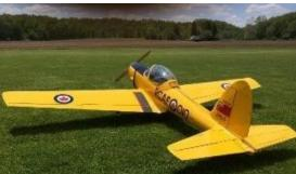
The plans include 6 sheets 36" x 80" with all parts and patterns shown. A cowl and canopy are available. Undercarriage is 5/8" diameter see page 44 Robart Robo-Struts. The wing is two-piece, plug-in type with the wing break just outside of the wing walk so the wing to fuselage fairings are constructed as part of the fuselage.
