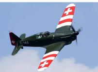
This is the Swiss version of the French M.S. 40 and M.S. 412. The most visible difference being a fixed engine coolant radiator.
