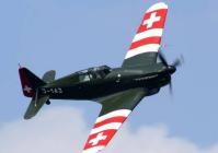
This is the Swiss version of the French M.S. 40 and M.S. 412. The most visible difference being a fixed engine coolant radiator.
